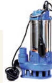
WQD15-15-1.5FA POWER: 1.5KW MAX FLOW: 416L/M MAX HEAD: 19M VOLTAGE: 220V SPEED: 2850RPM NET WEIGHT: 27KG
