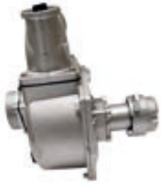
RK-PW-WP-D80 INLET & OUTLET SIZE: 3 INCH / 80MM FLOW MAX: 40 M3/H SUCTION: 7M DISCHARGE: 40M SPEED: 3600RPM PTO SHAFT SIZE: 18MM FOR GEAR DRIVE DIESEL MODELS
