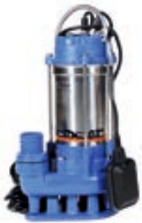
WQD10-11-0.75A POWER: 0.75KW MAX FLOW: 433L/M MAX HEAD: 14M VOLTAGE: 220V SPEED: 2850RPM NET WEIGHT: 18.5KG
